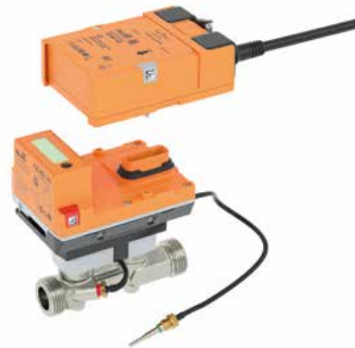
Figure 46: All wiring is to the logic module, allowing the EN1434/MID sensor module to be re-calibrated without disturbing the wiring
