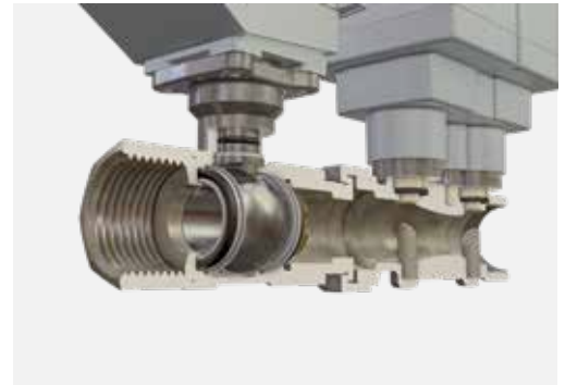
Figure 14: Electronic PI valves have a simple flow path, removing flow direction changes and significantly improving dirt tolerance
