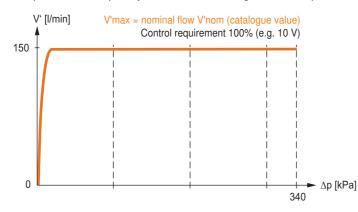
Pressure-independent flow over a large differential pressure range due to dynamic balancing (Example EP040R+MP)
