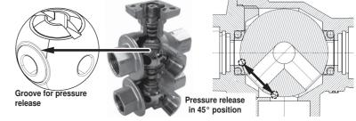
The corresponding differential pressure in the heating/cooling element is compensated for by means of the connection to the 'Sequence 1' circuit. After pressure compensation, there is no further water flow due to the same absolute pressures in Sequence 1 and in the heating/cooling element and the air-bubble tight closing lower closing element.
