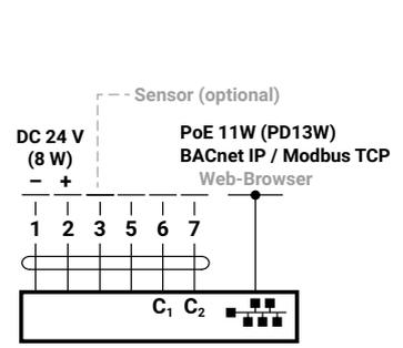
**PoE with BACnet IP or Modbus TCP with analogue output**
