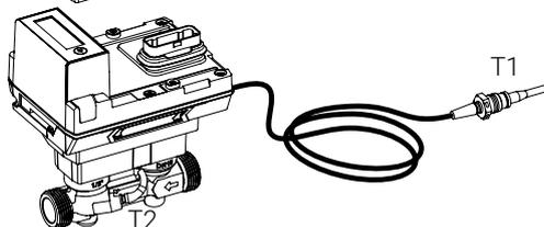
The thermal energy meter consists of a sensor module with connected temperature sensors, which houses the calculator unit and measuring system, and the logic module, which connects the thermal energy meter to the power supply and provides the bus and NFC communication interface. The sensor module is available as a spare part and must be replaced periodically for recalibration in certain countries according to national regulations.
