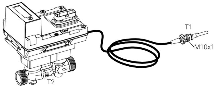
The connecting cable of temperature sensor T1 should not be laid along hot pipes or wound around them, as the wire resistance and its temperature dependency affect the measurement result of temperature sensors in two-wire technology.
