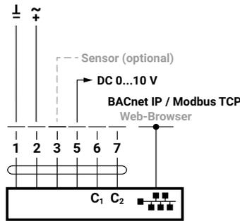
**PoE with BACnet IP or Modbus TCP**
