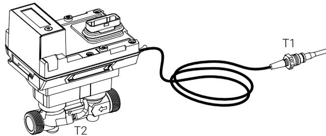
**Separate the logic module and sensor module**
