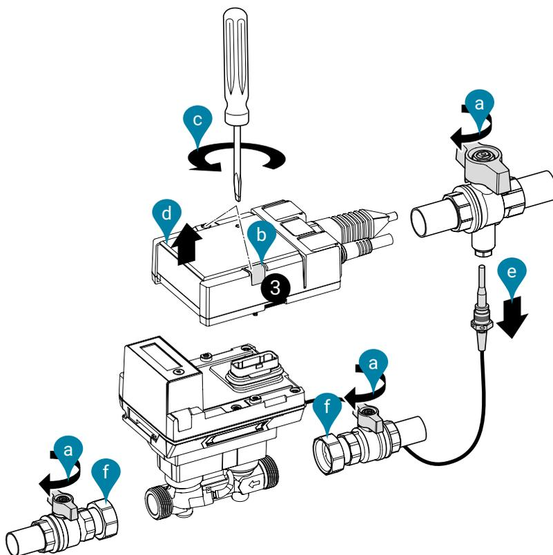
**Join the logic module and sensor module**
