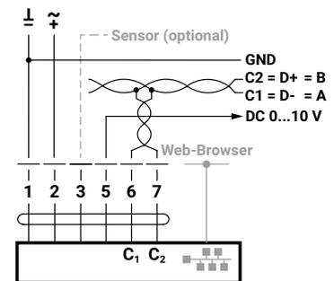
**Wiring BACnet MS/TP or Modbus RTU (daisy chain)**
