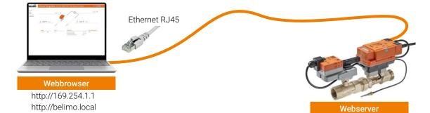
Note: The device must be supplied with voltage. If the device is powered via PoE, you can access the device only via the IP address or through the Belimo Assistant App.
