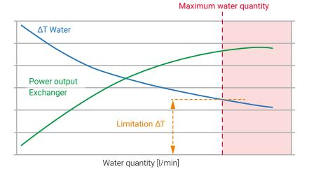
In operation, the limitation only monitors the differential temperature at a flow value  $\ge$ 30% of V'<sub>max</sub>.
