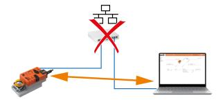
As an alternative to the link local address and "peer-to-peer" connection, you can also access the device using the IP address. This type of connection can also be used in a network with multiple consumers. If there are several devices in the network, valid IP settings have to be assigned to the consumers in advance (IP address and subnet mask).
